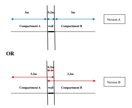
With clear indication, both Version A and Version B show the external dimensions of the two compartments clearly and the issue of "double-counting" will not arise.
